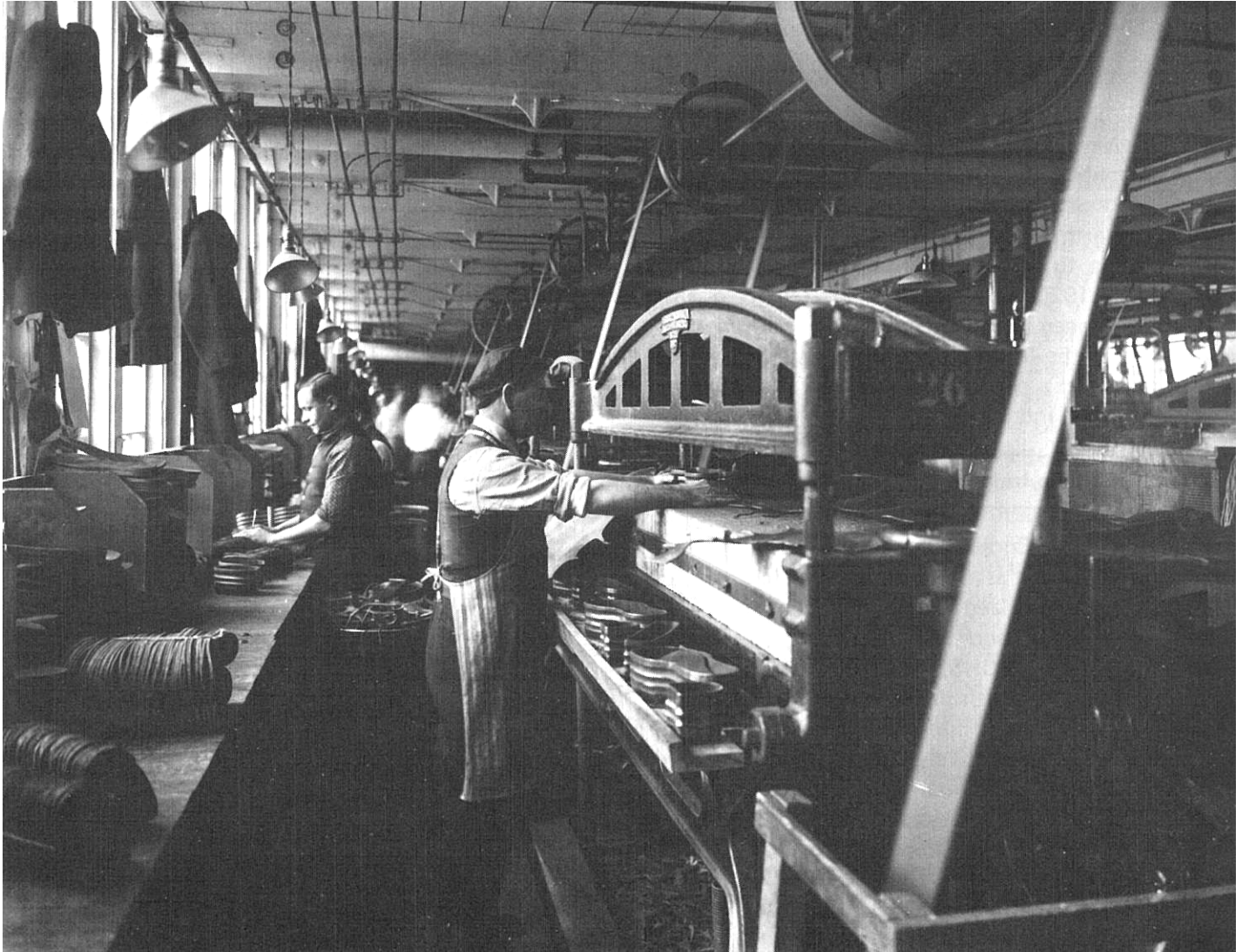
Figure B-31: Cutting soles and heels, Endicott-Johnson Company, Endicott, 1917 (from NYS Archives )
